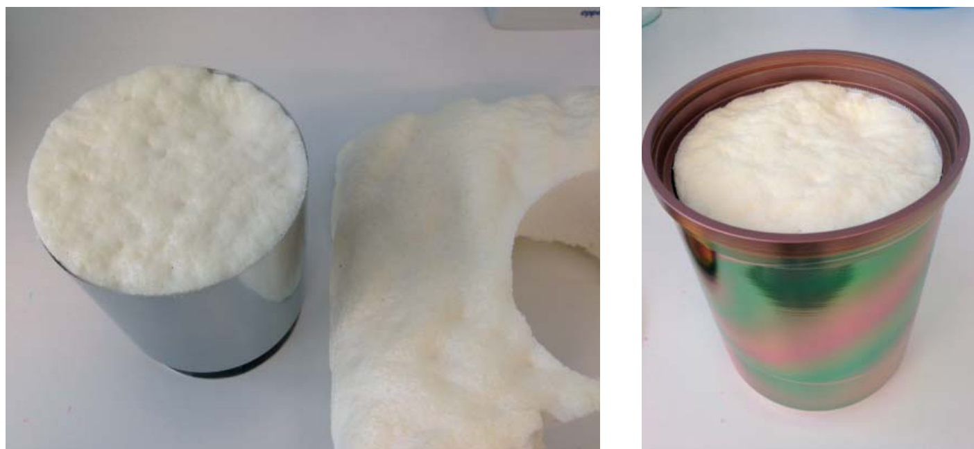
Figure 3. Custom-made coring tool and sample of the SPF open-cell foam (left) and the coring tool together with the sample, the surface at the top, placed into the one Liter container (right).
