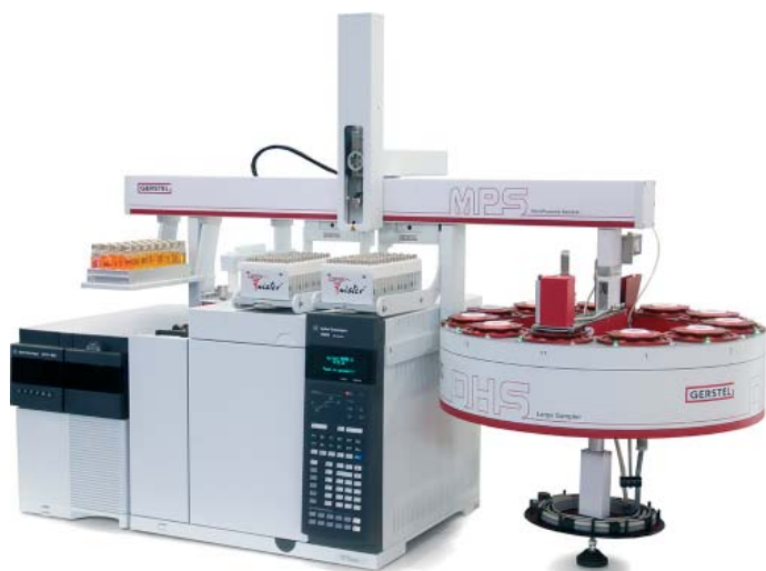
Figure 1. 11-Position on-line micro-scale chamber system coupled with TD-GC/MS.
